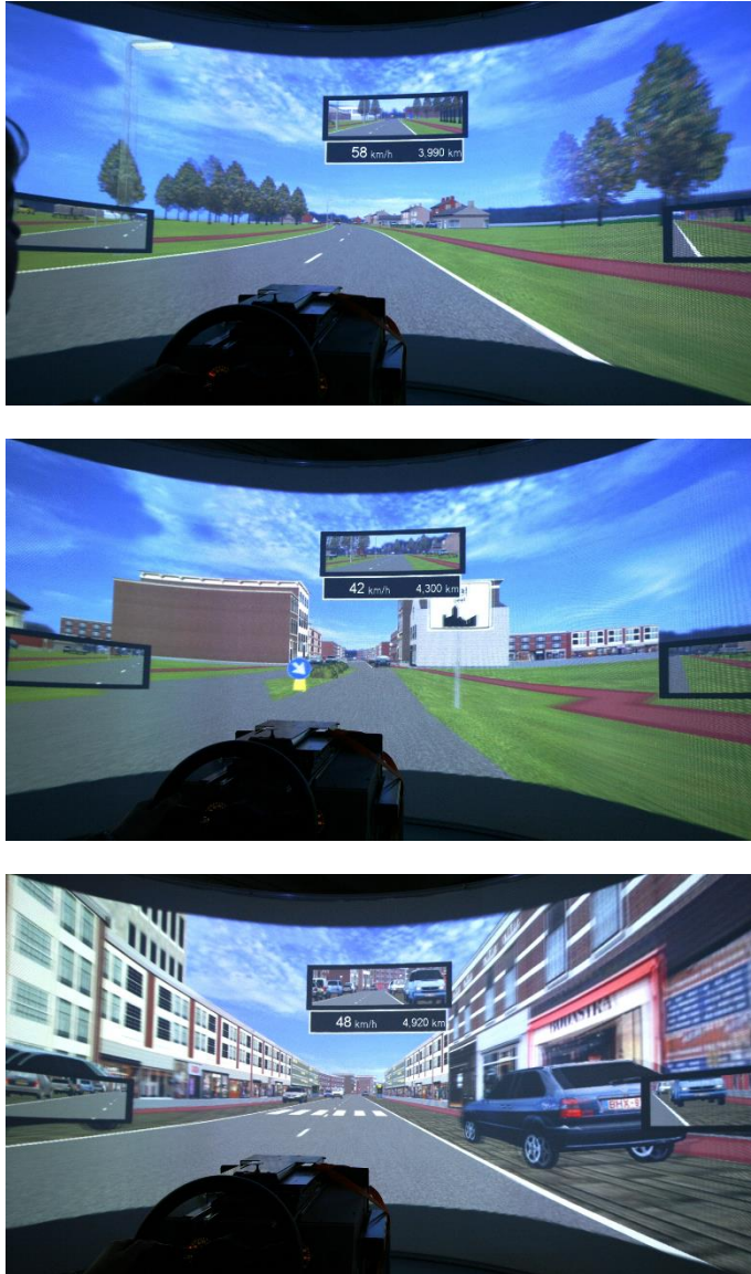
Figure 33 A simulator view of a rural road section, the rural-urban transition with gate construction and an urban area section
