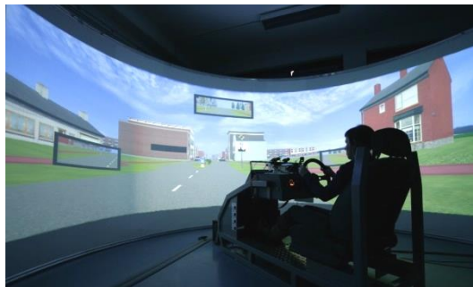
Figure 18 Medium-fidelity driving simulator at the Transportation Research Institute – Hasselt University
