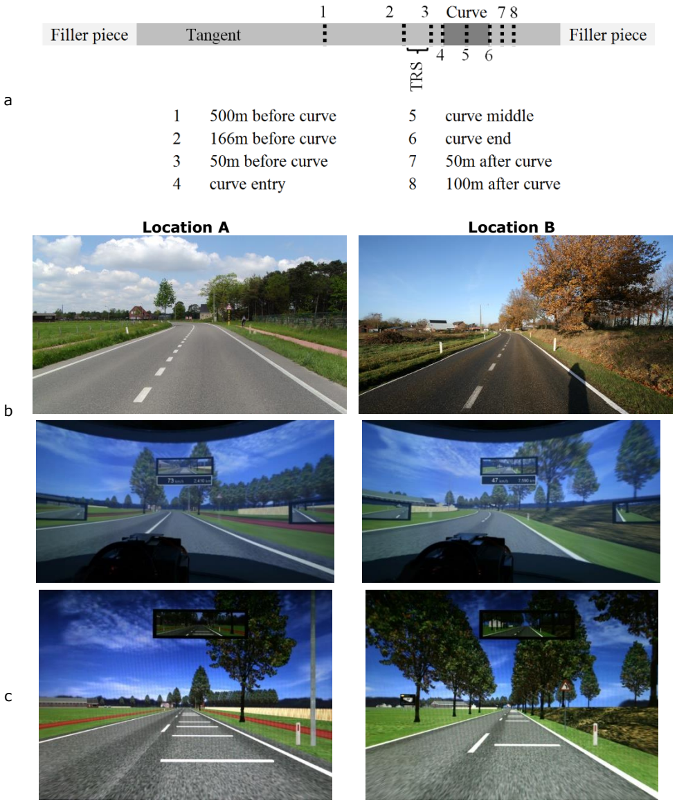
Figure 56 (a) Scenario overview; (b) real world versus simulator images nearby curves at location A (left) and B (right); (c) simulator images of TRS at location A (left) and B (right)
