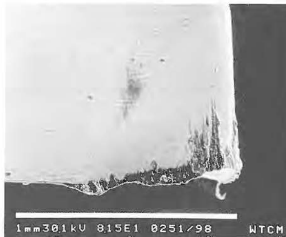
Fig.5 : Clearance face of a Hard Carbon coated WC-Co insert after 1,333min turning. Note the extent of abrasion and the formation of built-up edges.
