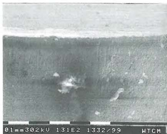
Fig.14 : Wear analysis showing little adhesion of aluminium on the clearance face of the tool after 90min dry machining of AlSi10Mg + 20wt% SiC ( v_c = 100\text{m/min} , f = 0.1\text{mm/rev} , a_p = 0.5\text{mm} ).
