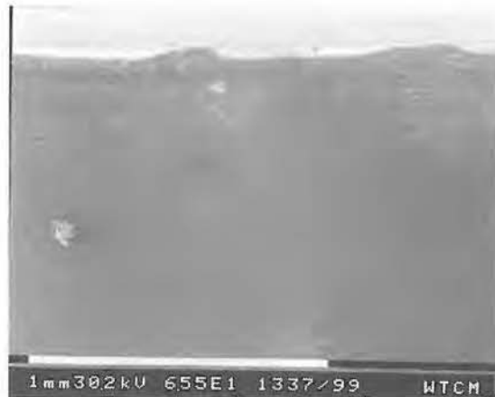
Fig.16 : Wear analysis showing adhesion of aluminium on the clearance face and formation of built-up edges on the cutting edge of the tool after 30min dry machining of AlSi10Mg + 20wt% SiC ( v_c = 200 m/min, f = 0.1 mm/rev, a_p = 0.5 mm).
