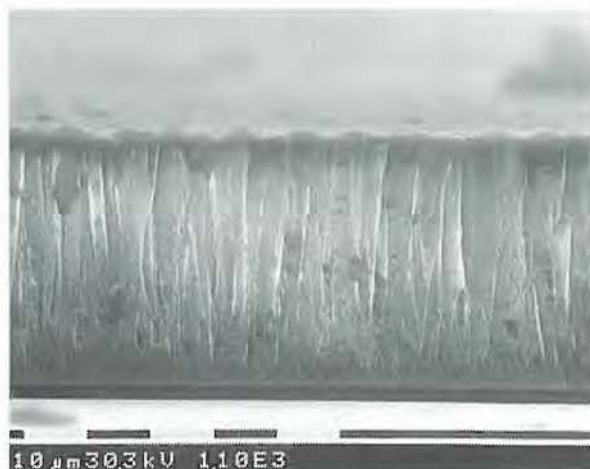
Figure 6.1: Columnar structure of the diamond growth film based on Van der Drift's principle of evolutionary selection [45].
