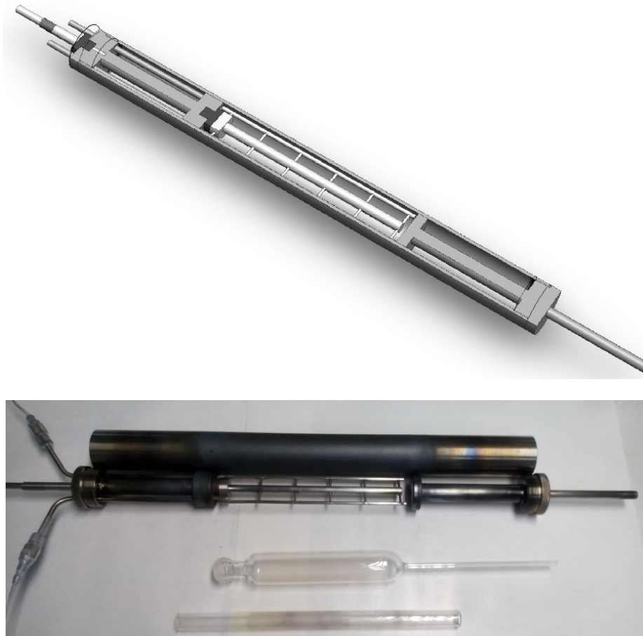
Figure 3-3: 3-D model pyrolysis and activation reactor (above), manufactured reactor in comparison with the quartz reactors (below).
