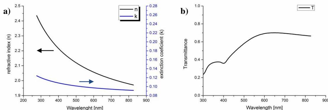
**Figure 2.** Dispersion of  $n$  and  $k$  (a) and transmittance (b) of diamond film measured at quartz slide.
