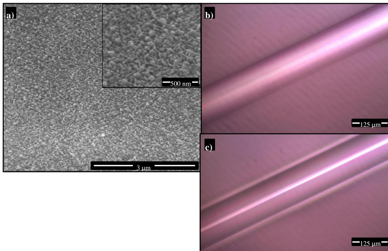
**Figure 1.** SEM image (a) and optical microscope image (b), (c) of diamond films on fused silica optical fibre.
