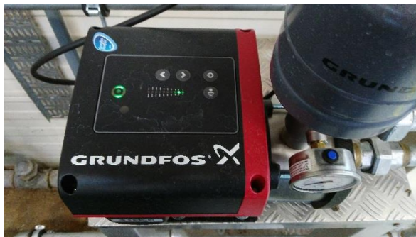
Pump on 2 nd power level for IPx5-testing (results in 12,5 l/min ± 5%)
