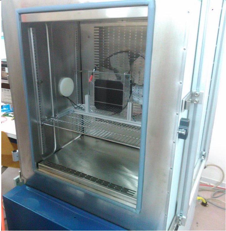
FIGURE 3-3: THE WEISS SB20 CLIMATE CHAMBER WITH A PV MODULE INSIDE READY TO MEASURE THE IV CURVE.
