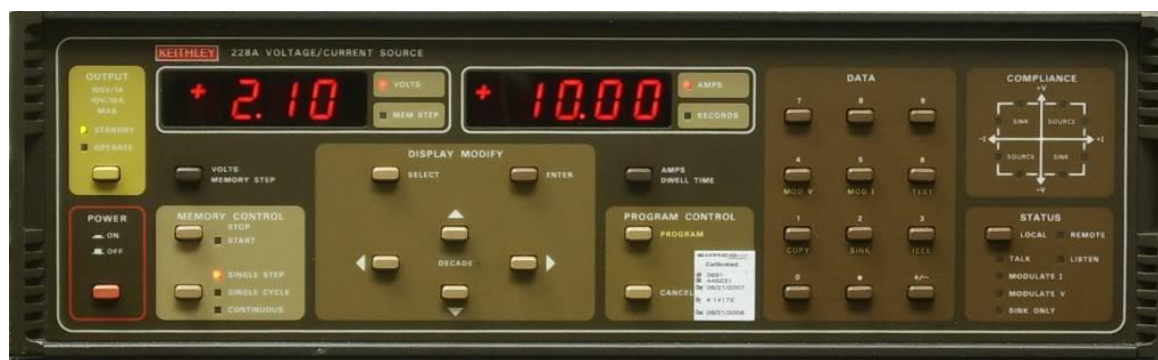
FIGURE 3-2: THE KEITHLEY 228A VOLTAGE/CURRENT SOURCE USED FOR MEASURING IV CURVES OF PV MODULES [36].
