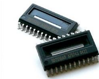
Figure 1 Picture of the package of the MLX75320 sensor product [2]
