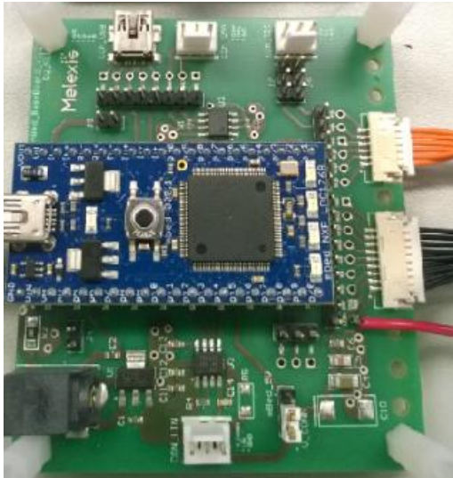
Figure 5 Picture of base board with mbed development board mounted
