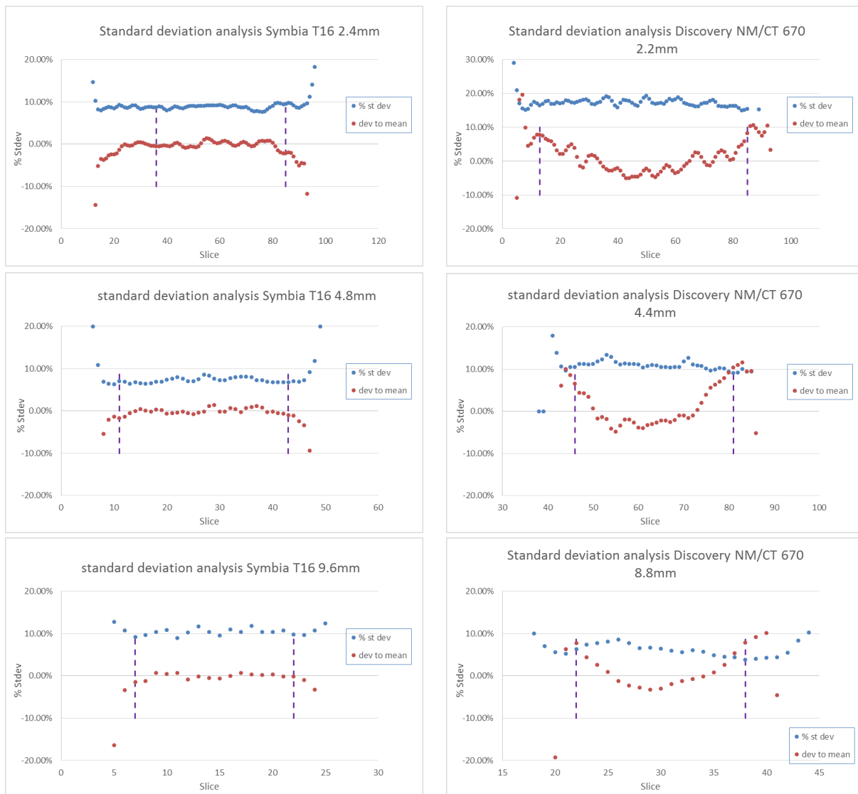
Figure 4.8: Standard deviation analysis of both imaging systems at different pixel sizes. Left: Symbia T16. Right: Discovery NM/CT 670
