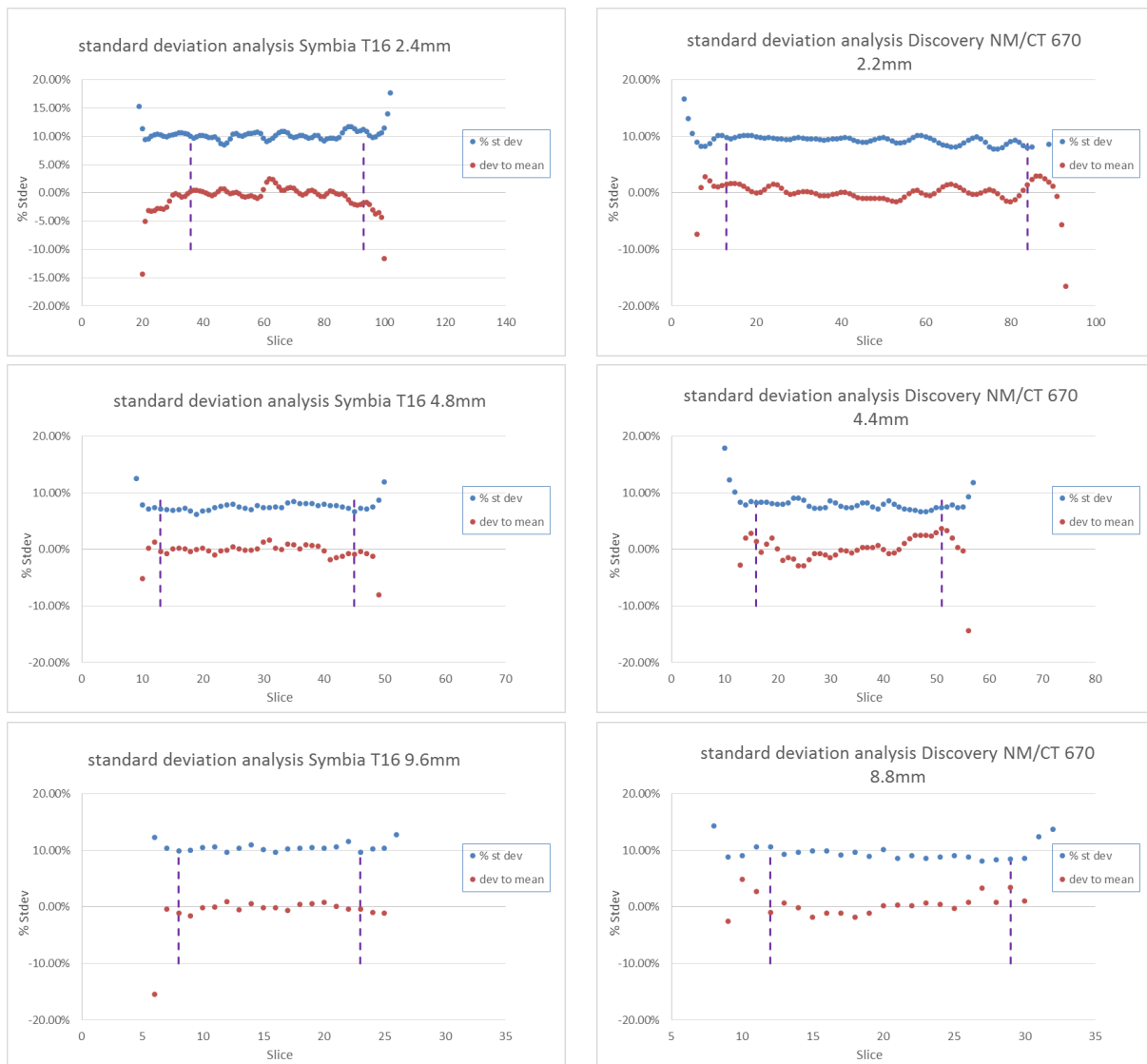
Figure 5.8: Standard deviation analysis of both imaging systems at different pixel sizes. Left: Symbia T16. Right: Discovery NM/CT 670 (reconstructed with Hermes Hybridrecon)
