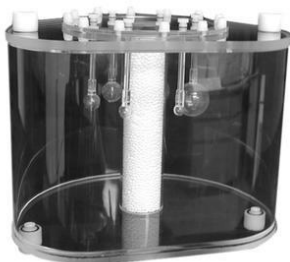
Figure 3.1: Illustration of the NEMA IEC body phantom. The lung insert in the middle left untouched [28]
