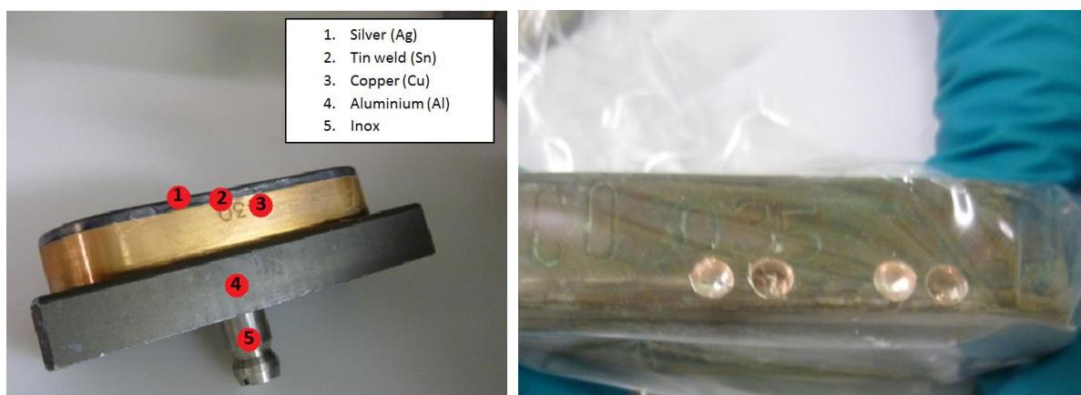
Figure 18 : sampling points (left), drill holes in target 'CO 035' (right)
