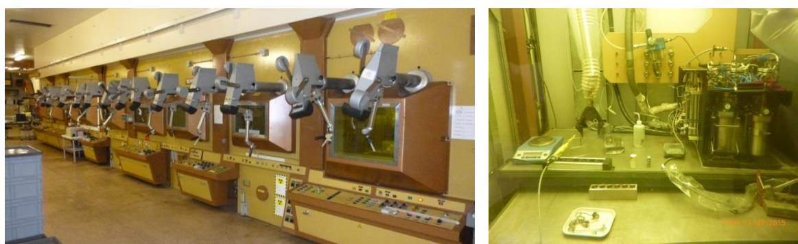
Figure 6: a) row of hot cells, b) content of cell C30
