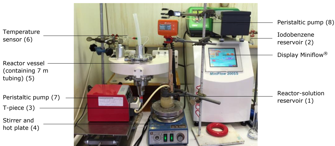
Figure 31: Microwave-assisted flow set-up
