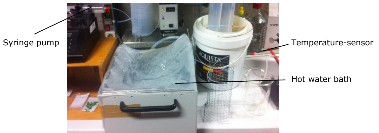
Figure 38: Experimental set-up for the determination of the overall heat-transfer coefficient
