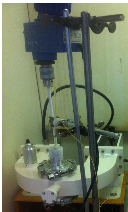
Figure 27: Overhead stirring set-up in the microwave reactor
