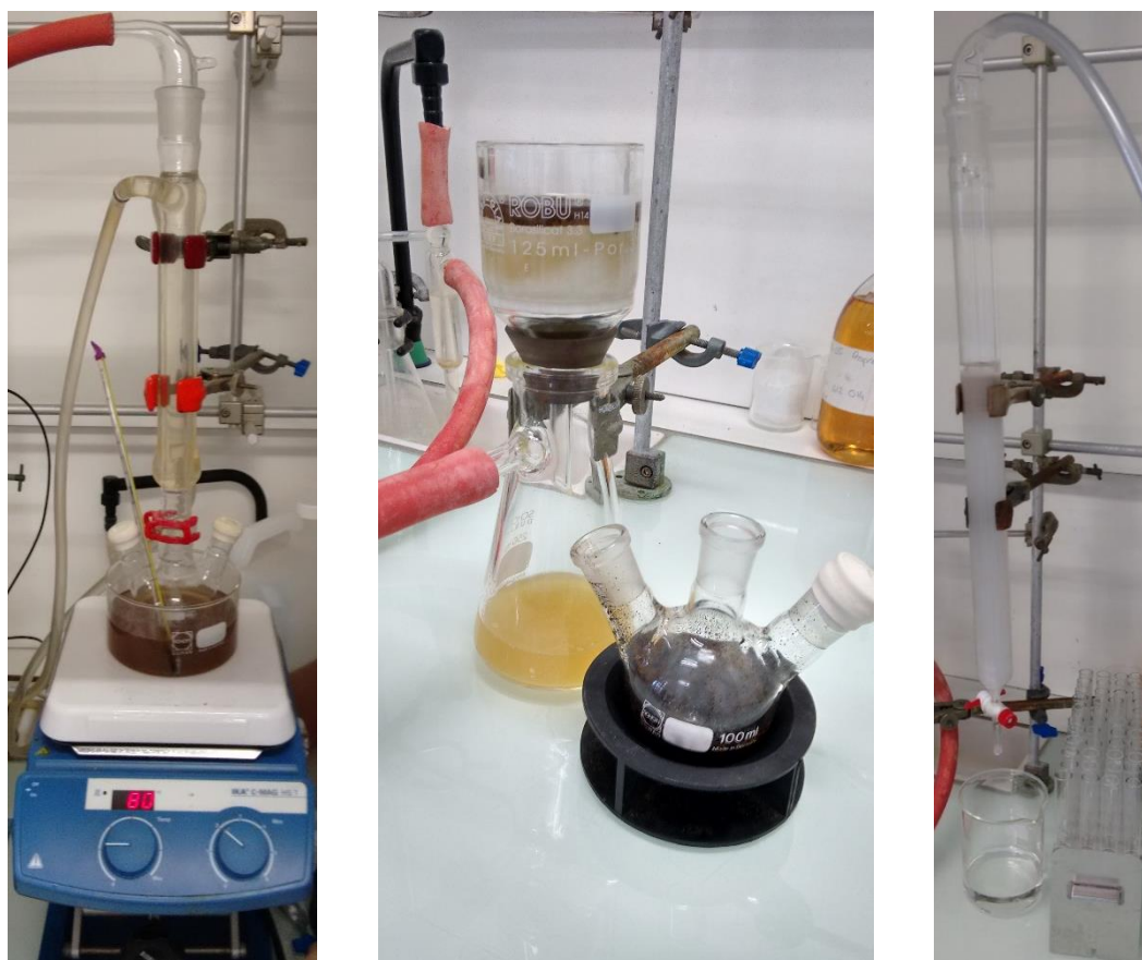
Figure 17: Setup of the Wittig reaction (left) and purification steps (vacuum filtration in the middle and column chromatography at the right).
