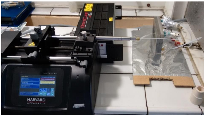
Figure 20: Setup of isomerization in flow.
