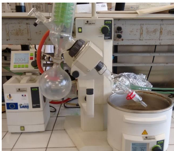
Figure 15: Rotary vacuum evaporator.
