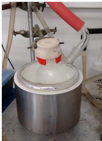
Figure 19: Degassing of the solution for flow trials.
