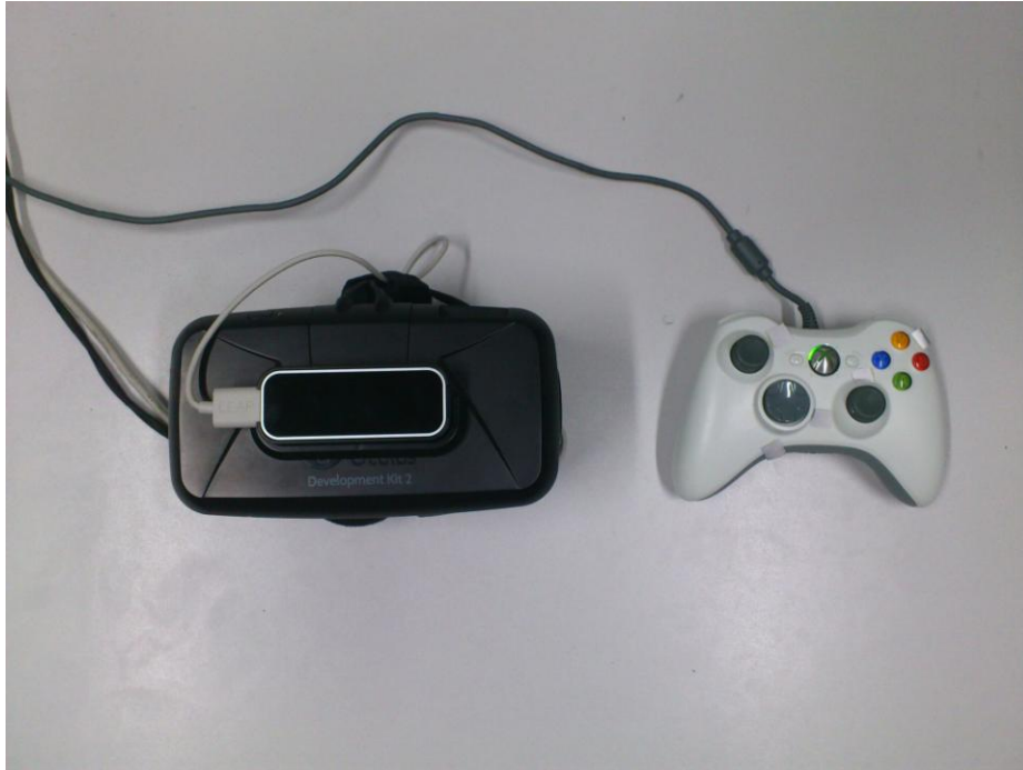
Figure 11: A possible hardware setup consisting of a Leap Motion mounted to an Oculus Rift Development Kit 2 and an Xbox 360 Controller marked with retroreflective stickers
