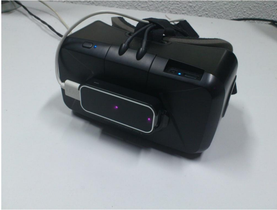
Figure 10: A Leap Motion mounted to an Oculus Rift DK2
