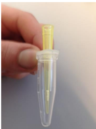
Figure 20. A stagetip column containing 3 layers of solid phase extraction disk in a 100 µl pipette tip. The tip was inserted into the microtube to collect fractions during purification.
