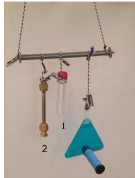
Figure 3 Hanging air exposure system for measurement of indoor concentrations of 1 : NO 2 and 2 : benzene and toluene (within the same tube).
