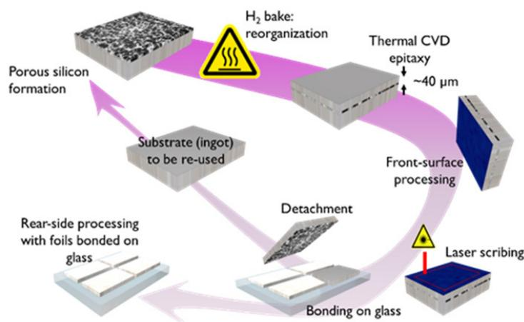
Fig. 1. i2-module concept using epitaxy for fabricating (thin) Si wafer material and cell processing while the foil remains attached to a carrier throughout the process
