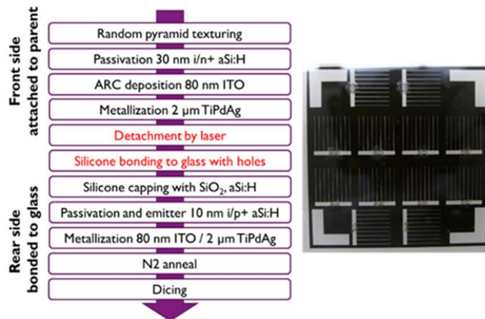
Fig. 5. Used process sequence for cell integration of the epifoils (left); front view of the resulting (12) cells before dicing (right), note the holes in the glass to contact the busbars on the front
