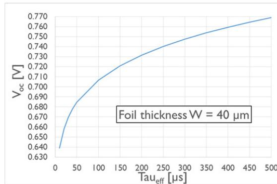
Fig. 6. Impact of effective lifetime on Voc, for 40  $\mu\text{m}$  thick Si foils
