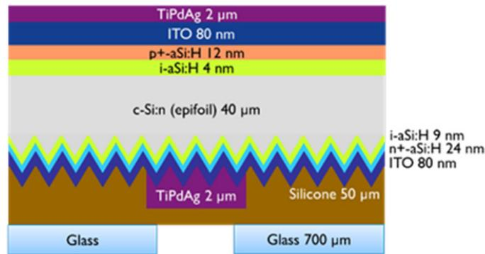
Fig. 4. Schematic cross-section of the cell buildup (not to scale); the front side glass facing the sun is drawn here at the bottom
