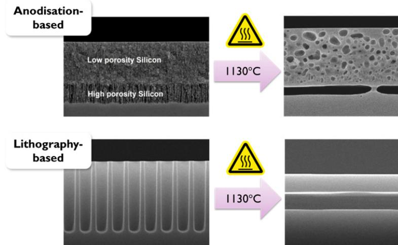
Fig. 2. Preparation of template material for epitaxy for 2 routes being used at imec to obtain (after detachment) thin wafers: based on anodisation (top) and on deep UV lithography (bottom)
