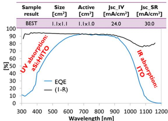
Fig. 7. Breakdown of Jsc losses: Jsc\_IV and Jsc\_SR respectively give the value measured by light IV measurement and derived by spectral response measurement (top table); parasitic absorption losses can be determined from comparison between EQE and (1-R) (bottom graph)
