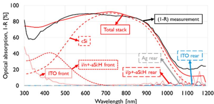
Fig. 8. Optical simulation indicating spectral per-layer-absorption for bonded flat cells, with comparison to measured value for (1-R)
