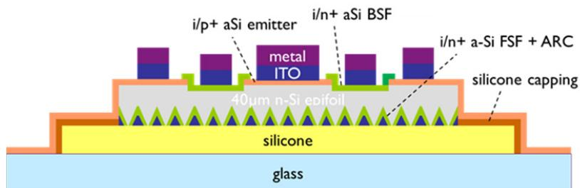
Fig. 10. Layout of IBC structure incorporating potential improvements.
