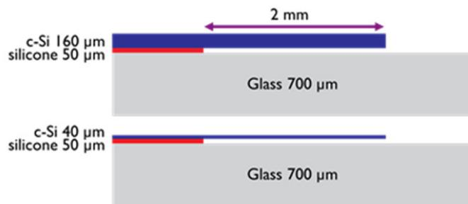
Fig. 3. Thinner wafers increase risk of breakage at fragile edges and increase issues with liquid trapping during wet processing
