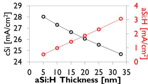
Fig. 9. Simulation for flat cells indicating impact of the thickness of the front i/n+-aSi:H on Jsc loss due to parasitic absorption in that layer
