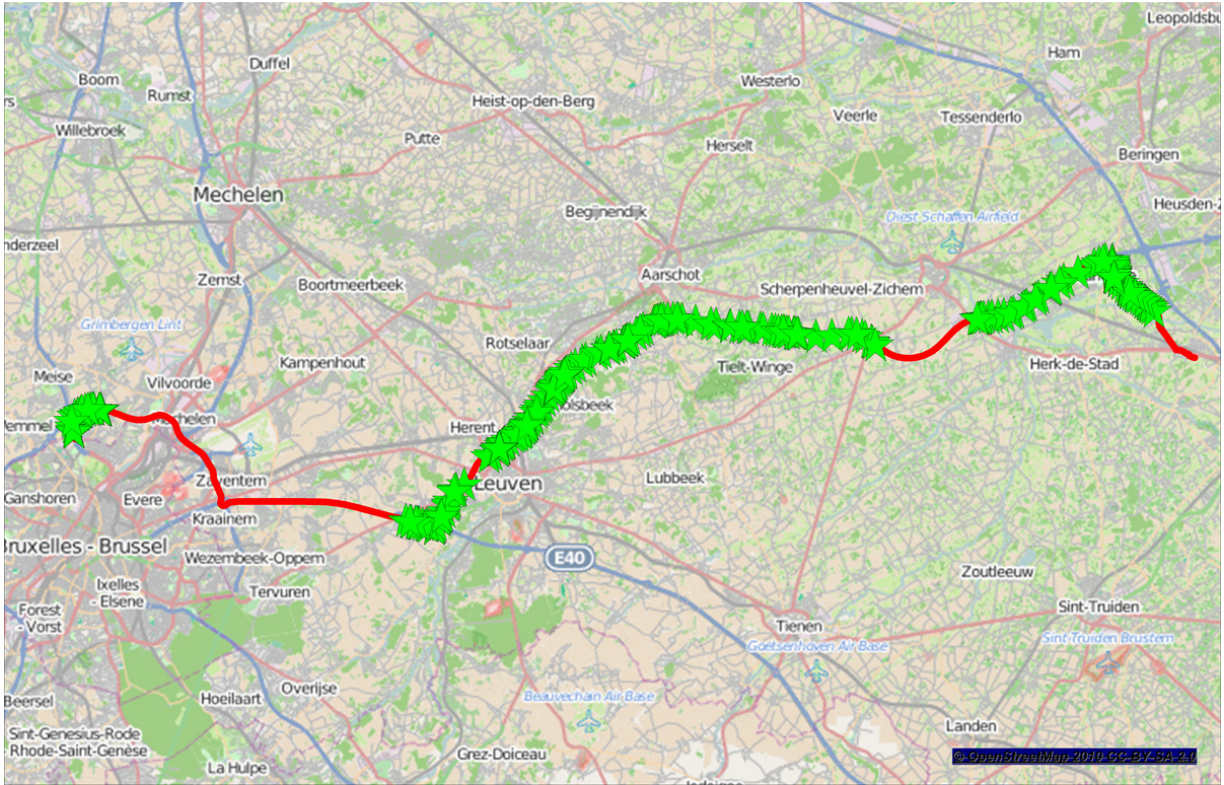
Figure 5: The largest part of the route (from Herk-de-Stad (right) to Kraainem (left)) makes use of the E314 and E40 highways. SplitVertices (represented by green star symbols) were determined using the raw (non-normalized) OSM network. The diagram shows the need for network normalization.
