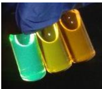
Figure S15. Fluorescence of P(3HT- alt -P) (left), P3HT- b -P(3HT- alt -P) (middle) and P3HT (right) in chloroform solution under a UV lamp at 365 nm.
