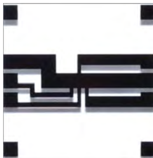
Figure 5.2: Depiction of a nanocrystalline diamond film on glass patterned into a Hall bar structure.
