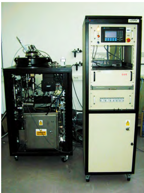
Figure 2.3: Picture of the ASTeX 6500 reactor as installed at IMO.
