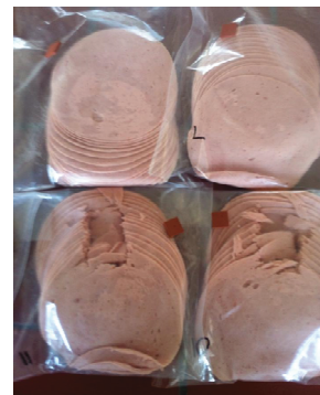
Figure 4: Discoloration in defective pouches (above) and preservation of colour in intact pouches (below) of sliced ham sausage (day 20)
