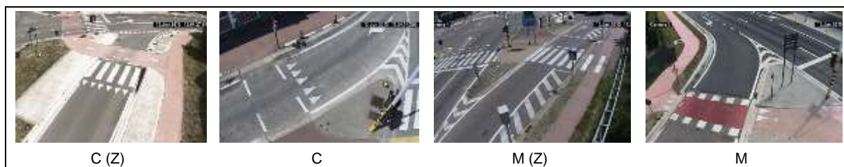
Figure 2: Screenshots from the cameras closest to the crossing facilities at the four locations. Locations are named based on priority rule (cyclists (C) or motorists (M) have the right-of-way) and the presence of a zebra crossing (Z).
