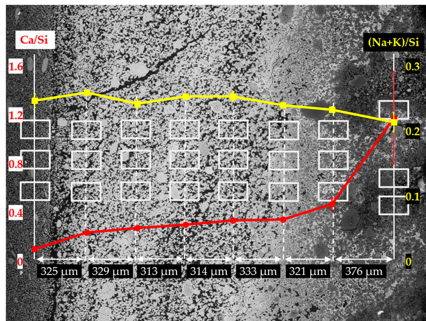
Figure 16. Changes of Ca/Si ratio and (Na+K)/Si ratio of the areas from the sample reacted for seven days. The red curve represents the change of Ca/Si ratio, the yellow curve represents the change of (Na+K)/Si ratio.
