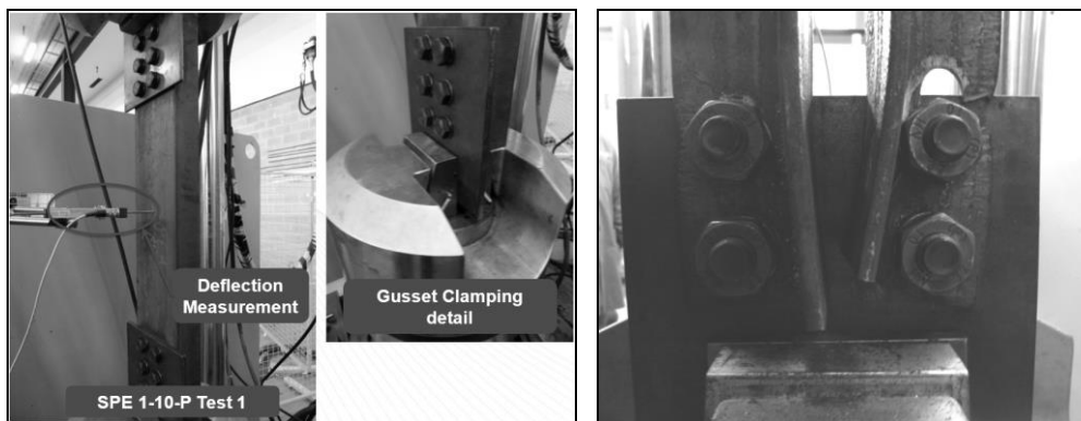
Figure 1. Test setup and example of failure mode.
