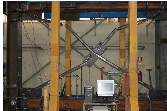
b. After both bracings completely fractured
