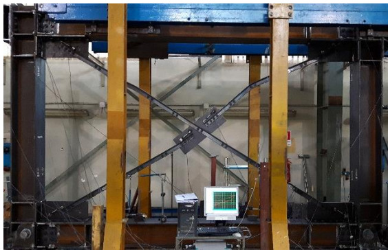
a. During post-buckling
