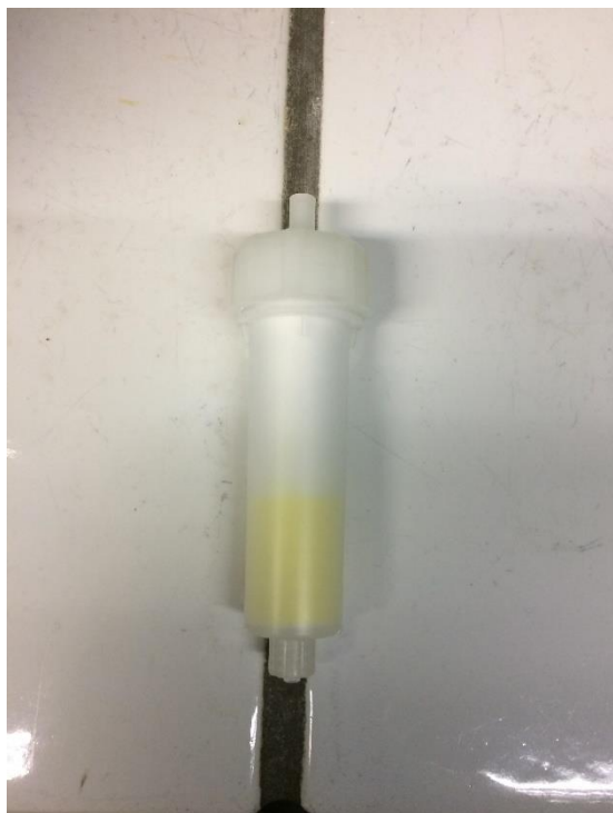
Figure S6.1. Pictures of the Büchi sepacore system equipped with GRACE Resolve normal phase silica cartridges (40 gram). Left) Crude oligomer mixtures were embedded on silica and loaded into a pre-column cartridge and placed on top of the GRACE resolve normal phase silica cartridges. Right) Picture of the Büchi sepacore setup during oligomer separation.
