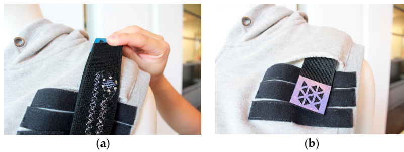
Figure 6. Garment Implementation: (a) Sensor embedded in a Velcro strap by coated conductive yarn; (b) Velcro adjustments.
