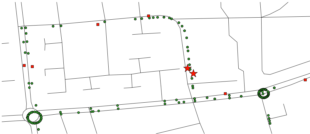
Fig. 1: Israel, Kiryat Gat: example of inaccuracy. Shapes (green circles) and bus stops (red squares/stars) in GTFS displayed on an OSM network. The stops represented by the red stars show the wrong side of the road problem. Note the missing roundabout at the right side and the positional errors.
