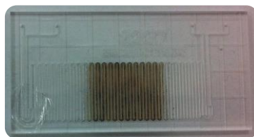
Figure 1.9. Example of a clogged Labtrix® 3227 reactor.
