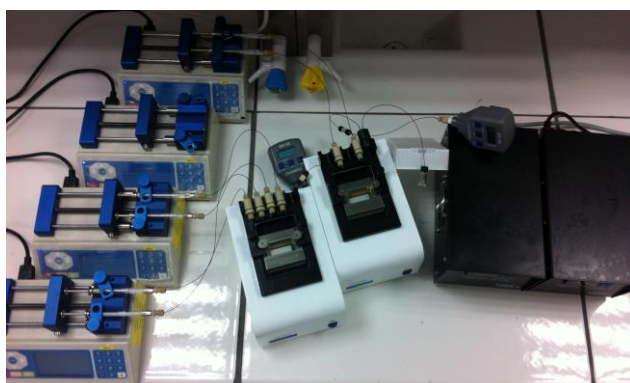
Figure 7.2. Microreactor cascade as used for the triblock copolymerizations.
