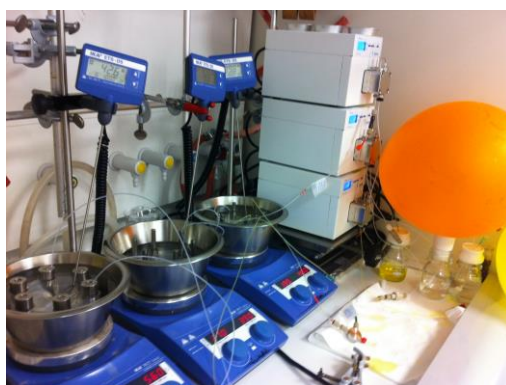
Figure 7.4. Representation of the [0.8 mL + 3.6 mL + 5.2 mL] tubular reactor cascade, employed for triblock copolymerizations.
