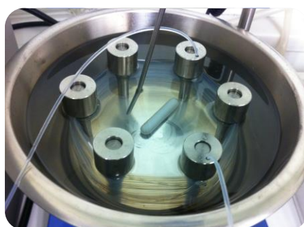
Figure 1.7. Tubular reactor, with reactor channels of 0.75 mm inner diameter.
