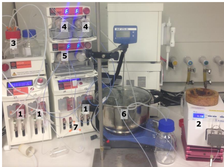
Figure S3. Modified Syrris Asia continuous flow set-up: syringe pumps (Syrris Asia; 1 ), Knauer AZURA P2.1S HPLC pump ( 2 ), solvent reservoir bottles ( 3 ), injectors (5 mL; 4 ), solvent switcher ( 5 ), 11.6 mL tubular reactor ( 6 ), and T-piece mixer ( 7 ).
