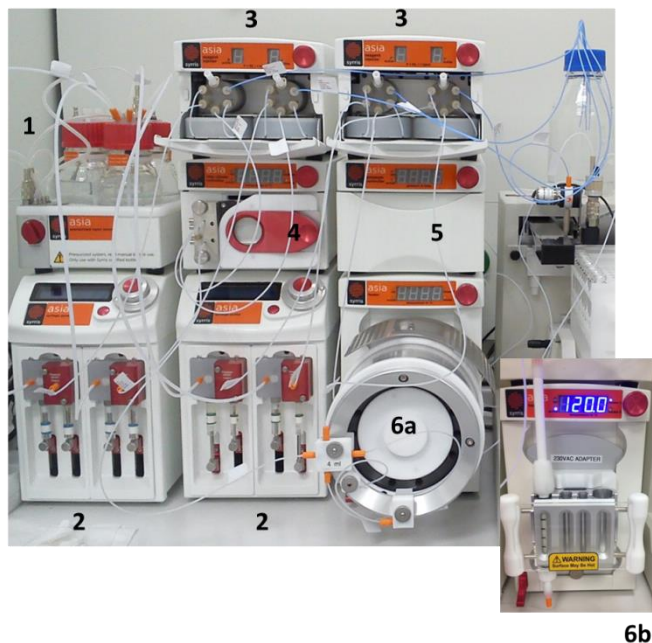
Figure S1. Syrris Asia 320 system: 1. Pressurized solvent/reagent input store; 2. Dual pair syringe pump; 3. Reagent injector with 5 or 10 mL PTFE loops; 4. Glass chip heater (0.25–1 mL glass chips; temperature up to 150 °C); 5. Back pressure regulator (BPR); 6. Heater module with adaptor for a) tubular or stainless steel reactor (4–16 mL) and b) solid-phase reactor.
