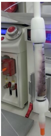
Figure S3. Bad elution of the reagents through the solid-phase reactor when using \text{CH}_3\text{CN} or THF as a solvent for the N-alkylation reaction of 6-Br-isatin ( 2 ).
