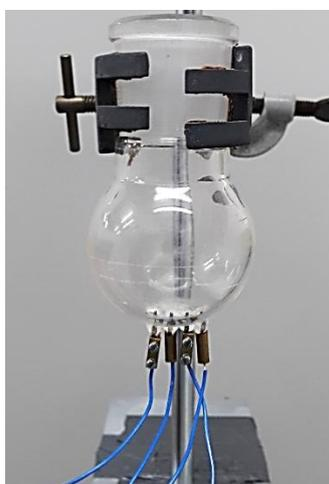
Figure 29: Round bottom flask with built-in electrodes and Teflon wires
