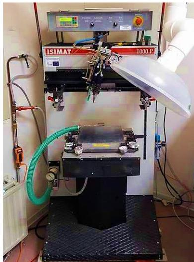
*Figure 14: Screen printer with ventilation (IMO-IMOMECE)*
