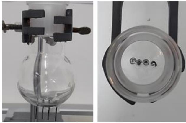
Figure 24: Round bottom flask with built-in tungsten electrodes: (left) front view, (right) top view
