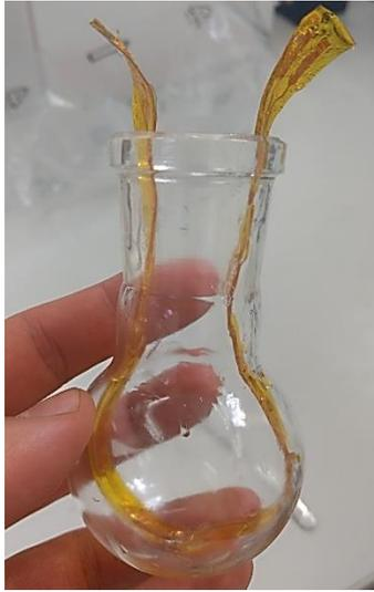
*Figure 23: Handmade measuring electrode in round bottom flask*
