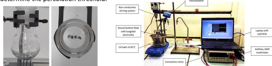
Figure 1: Design of round bottom flask with built-in tungsten electrodes (left); measurement set-up (right)
