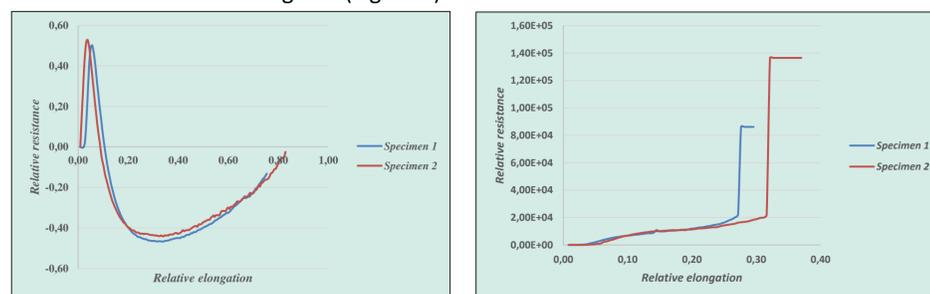
Figure 4: Relative resistance as a function of relative elongation: cylindrical particles (left); spherical particles (right)
