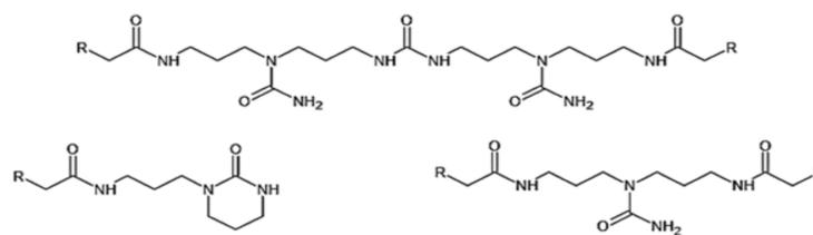
Figure 3: Structural formula of self-healing mixture
