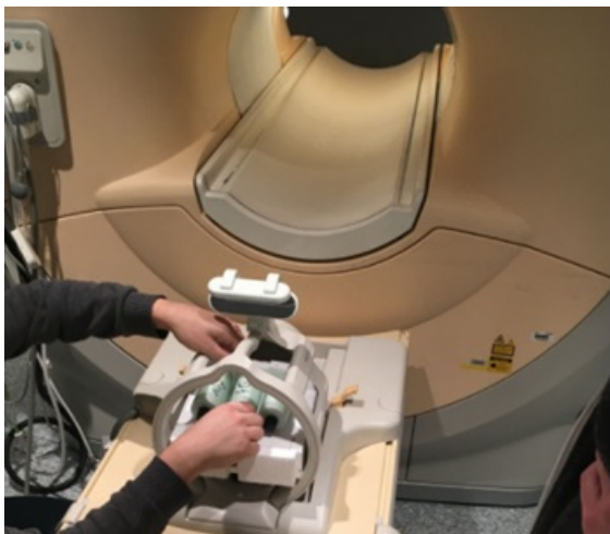
Figure 4.1: Read-out set-up for cuboid A and B: prints and calibration vials were surrounded by a styrofoam construction and put in a 8-channel head coil.
