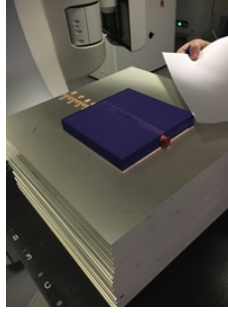
Figure 3.2: The set-up: a printed cuboid on 20 water-equivalent RW plates.
