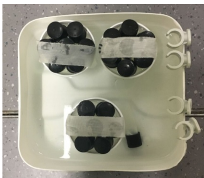
Figure 5.4: Scanning set-up for the calibration vials. The water tank was also placed in a 8-channel head coil.
