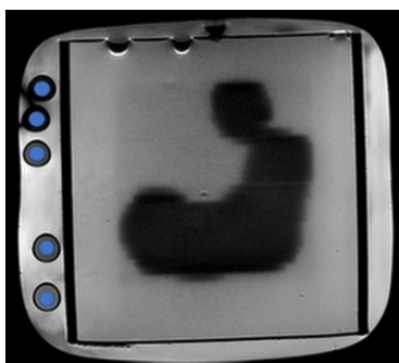
Figure 5.5: Echo of a MRI slice from cuboid A. ROI for acquisition of the mean R_2 and standard deviation are coloured in blue.
