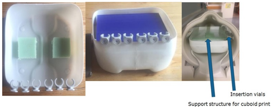
Figure 5.3: Read-out set-up for run 2: each cuboid was placed onto the support structures and completely surrounded by water doped with contrast liquid. The calibration vials were inserted next to the cuboid in the provided holders. Eventually the construction was placed in a 8-channel head coil which would be inserted in the MRI imager.
