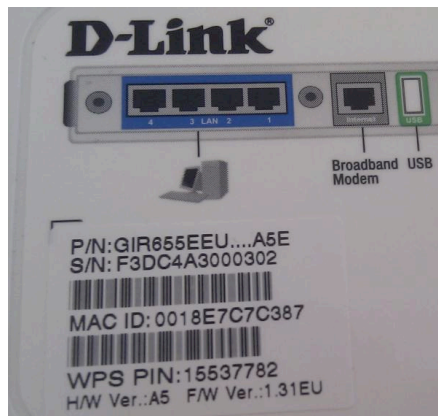
Figure 3.1: Label with WPS PIN on the back of a D-Link router [5: p.4]
