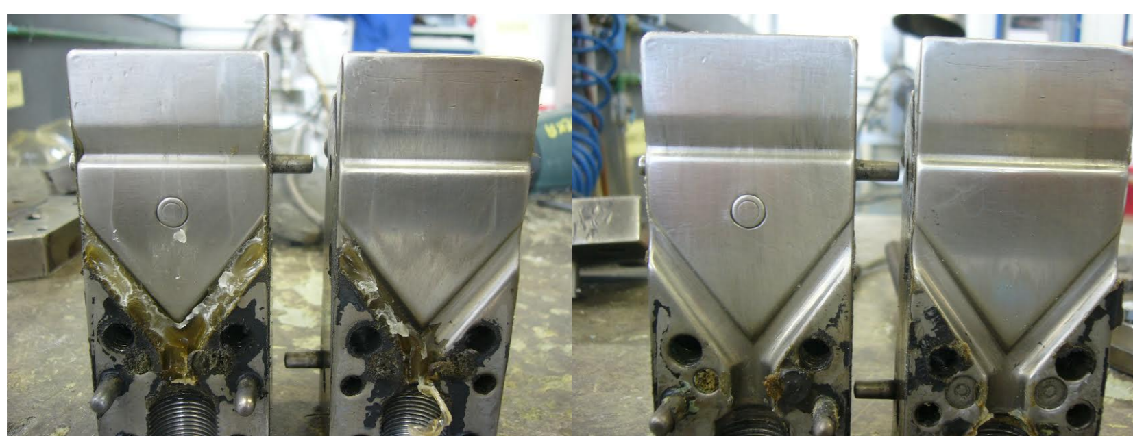
Figure 2: Example of a die with plate-out (left) and without plate-out (right)
