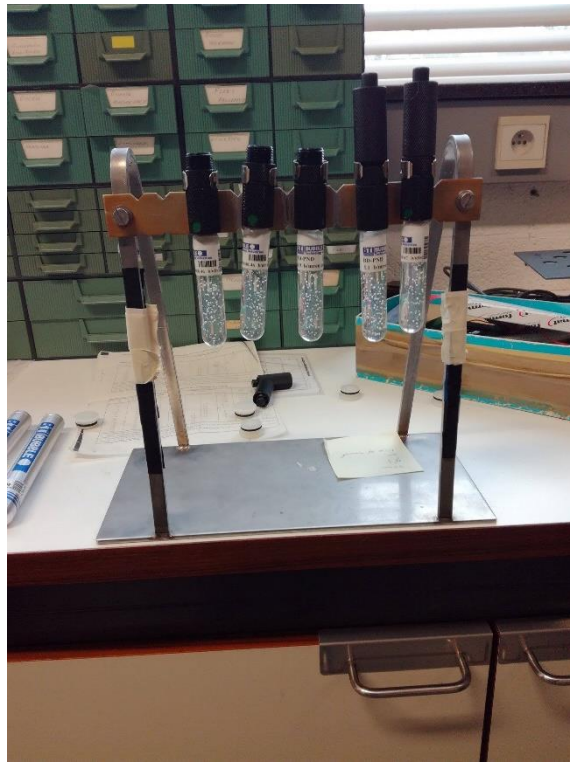
Figure 34: Irradiated BD-PNDs, the detectors were in the beam together on the small rack.
