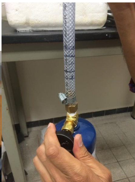
Tube connected to R227 container
