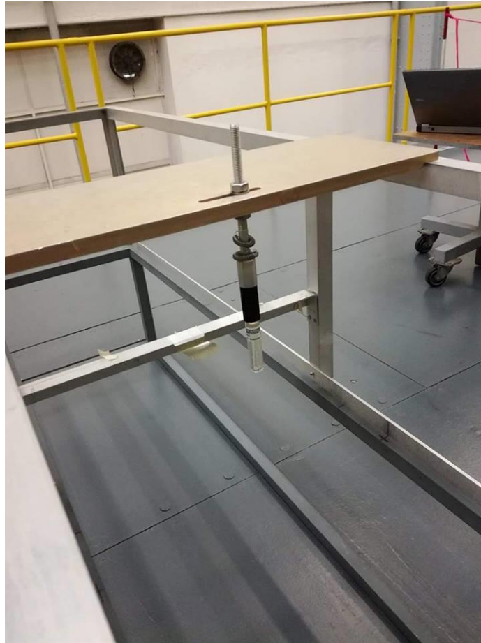
Figure 36: Bubble detector holder with BDT in the aluminum construction at channel Z55.
