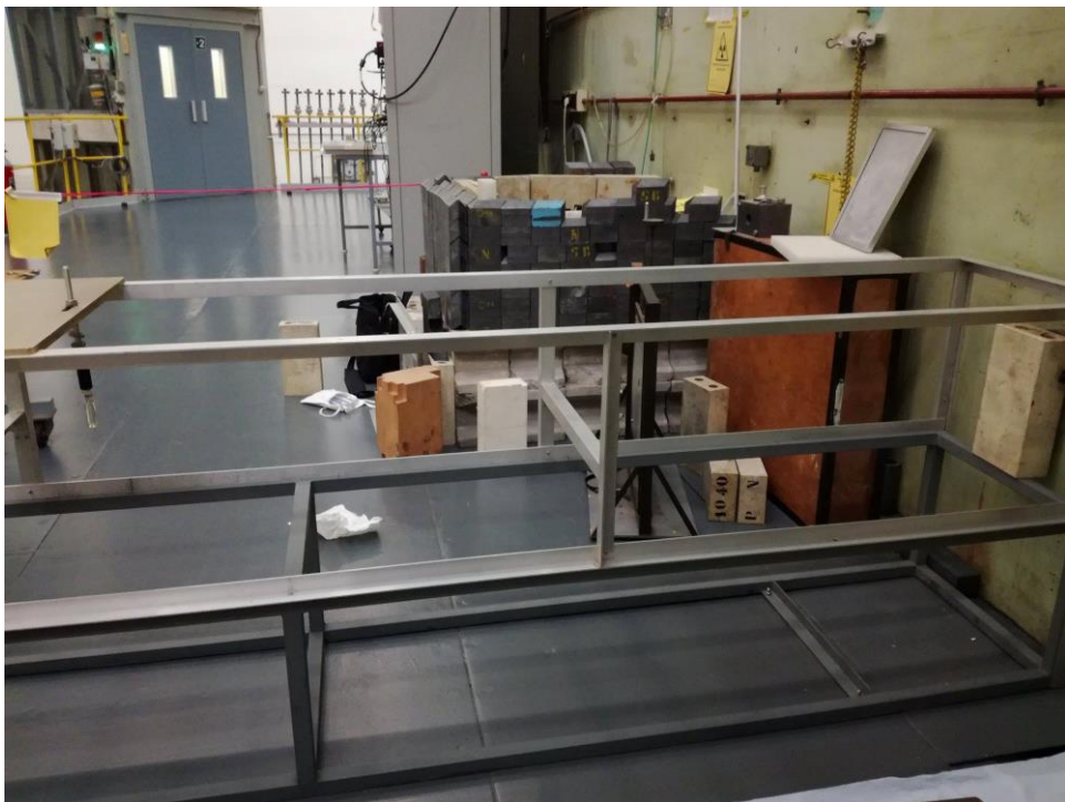
Figure 35: Irradiation set-up for the bubble detector BDT at channel Z55.
