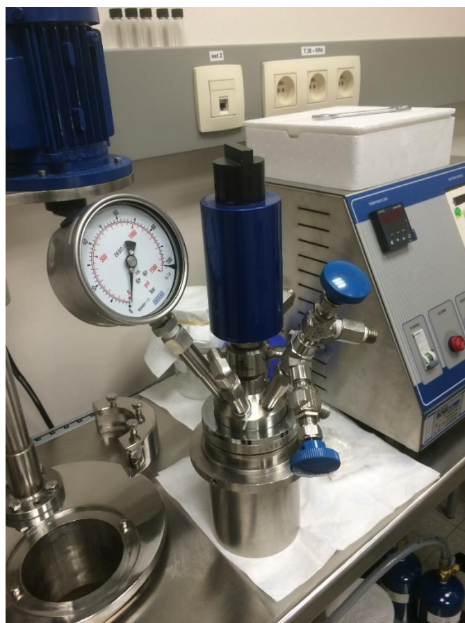
Figure 11: Pressure reactor with aluminum container.
