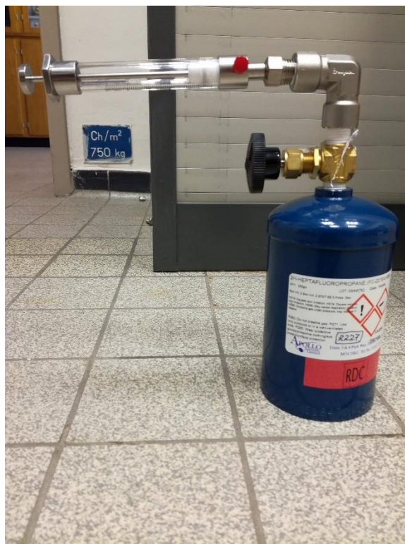
Figure 14: Gas syringe connected to the Freon container.
