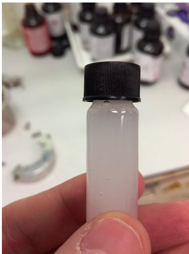
Figure 15: Self fabricated SDD.
