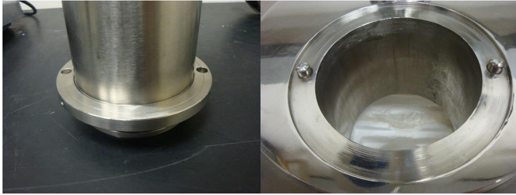
Holes on the sides of the aluminium container Bulges on stirring installation to fit with holes
