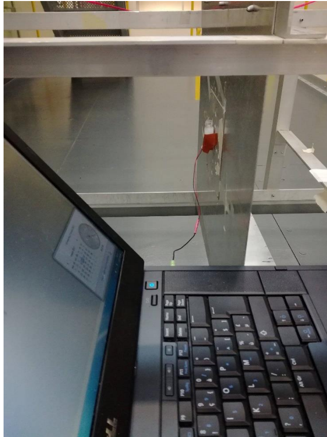
Figure 33: SDD taped to a metal plate in connection with a laptop at channel Z55B.
