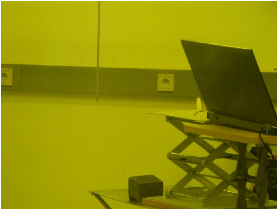
Figure 31: Neutron source at the end of the rod (left-hand side) and the SDD on the right resting on a piezoelectric microphone connected with a laptop.
