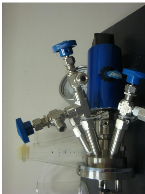
On the left hand you can see the part with 2 inlets and 2 valves (DIP TUBE)
