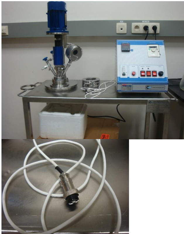
Stirring installation with temperature probe
