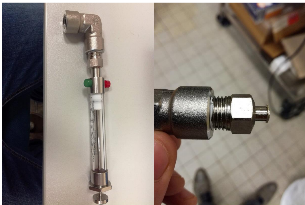
Figure 13: Gas syringe Pressure-Lok Serie A-2 from VICI Precision Sampling (left-hand side) and the elbow and coupler (right-hand side).
