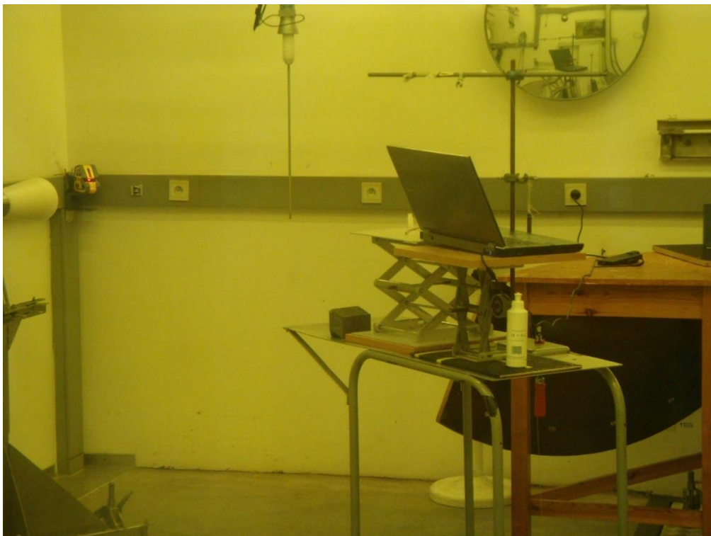
Figure 30: Calibration set-up, including the SDD, a laptop installed with the LabVIEW program and the CF3 source.
