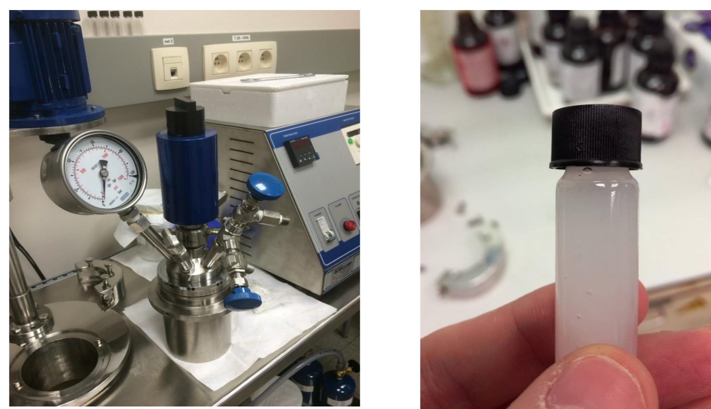
Figure 2: Pressure reactor (left-hand side) used to fabricate the gel for the SDD (right-hand side).
