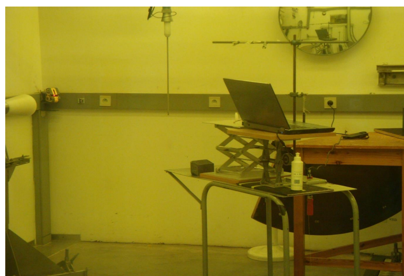
Figure 3: Calibration set-up, including the SDD, a laptop installed with the LabVIEW program and the ^{252}\text{Cf} source at the end of the rod.
