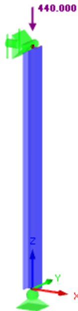
Figure 40: RFEM graphic representation of the column GH.
