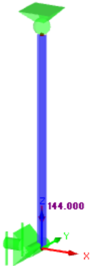
Figure 31: RFEM graphic representation of the steel tie.
