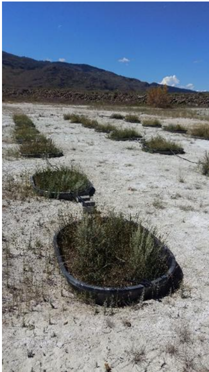
Figure 1: Ongoing experiment using nurse plants and soil additives to encourage plant growth on alkaline tailings
