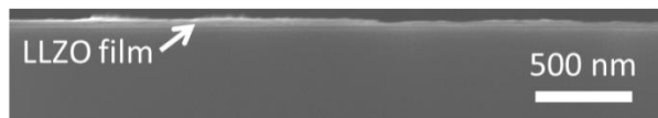
Figure 10: SEM (BSE) micrograph of LLZO film (30 to 60 nm thick) on a monocrystalline GGG substrate in the 111 orientation, as a results of 10 spray deposition cycles with the all-citrate Li-La-Zr-precursor (10 mM), with a deposition temperature of 200°C. The sample was submitted to a post-deposition anneal at 800°C for 4 hour in oxygen.
