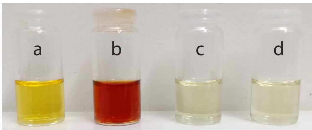
Figure 6: Photograph showing from left to right solutions of: (a) \text{Fe(III)(NO}_3)_3 , (b) \text{Fe(III)(NO}_3)_3 + KSCN, (c) \text{Fe(III)(NO}_3)_3 + ascorbic acid, (d) \text{Fe(III)(NO}_3)_3 + ascorbic acid + KSCN. Sample (b) shows the typical deep-red color of the \text{Fe(III)(SCN)}_3 complex, which forms in the presence of free \text{Fe}^{3+} . In sample (d), which in addition also contains ascorbic acid, no such color is observed, indicating that the \text{Fe}^{3+} is already reduced to \text{Fe}^{2+} .
