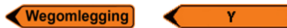
Figure 7: General temporary “detour” sign (left) & Specific temporary sign with municipality name “Y” (right)
