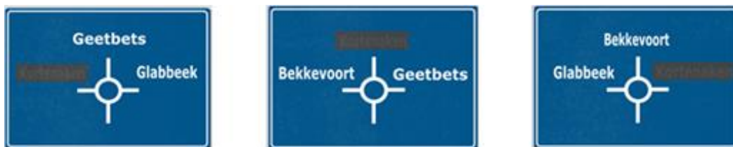
Figure 4: Regular blue advance direction signs with taped direction placed 200 m in front of the roundabout (left: southern branch; middle: eastern branch; right: northern branch)
