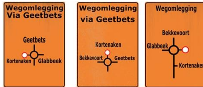
Figure 2: Specific temporary signalization at each branch (left: next to the temporary traffic light at southern branch (in front of the roundabout); middle: next to the temporary traffic light at eastern branch (in front of the roundabout); right: 100 m in front of the 3-way intersection at the northern branch (heading to the roundabout))
