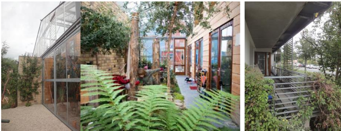
Figure 2: Pictures of some listed combined measures: {microclimatic space + greenery} (left and middle, 'EVA-Lanxmeer' / 'Serrewoningen' in Culemborg, The Netherlands), {sun-protection louvres + greenery} (right, 'Kronsberg' / 'Wohnanlage' in Hannover, Germany). (left and right: photo by Bart Janssens, 2012; middle: photo by Graphic alert)
