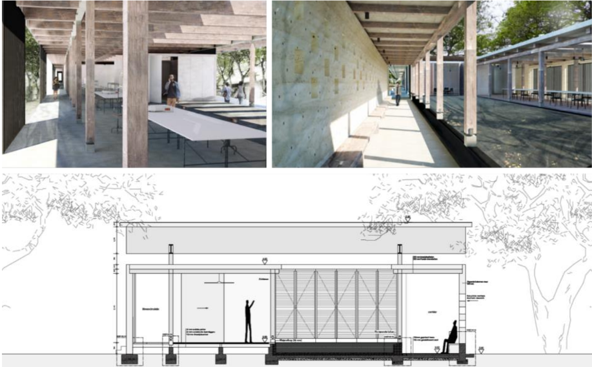
Figure 6: Student work on the Living Lab on university campuses, displaying a design (visualizations and section plan) for a new multifunctional pavilion.
