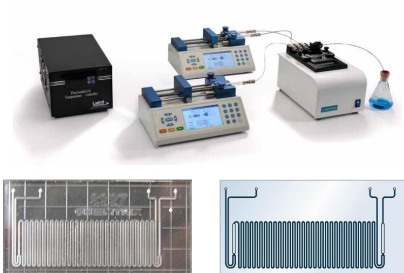
Figure 1.7. (top) Commercially available Labtrix® Start set-up and (bottom) Microreactor chip (19.5 \mu\text{L} ) utilized throughout this thesis.
