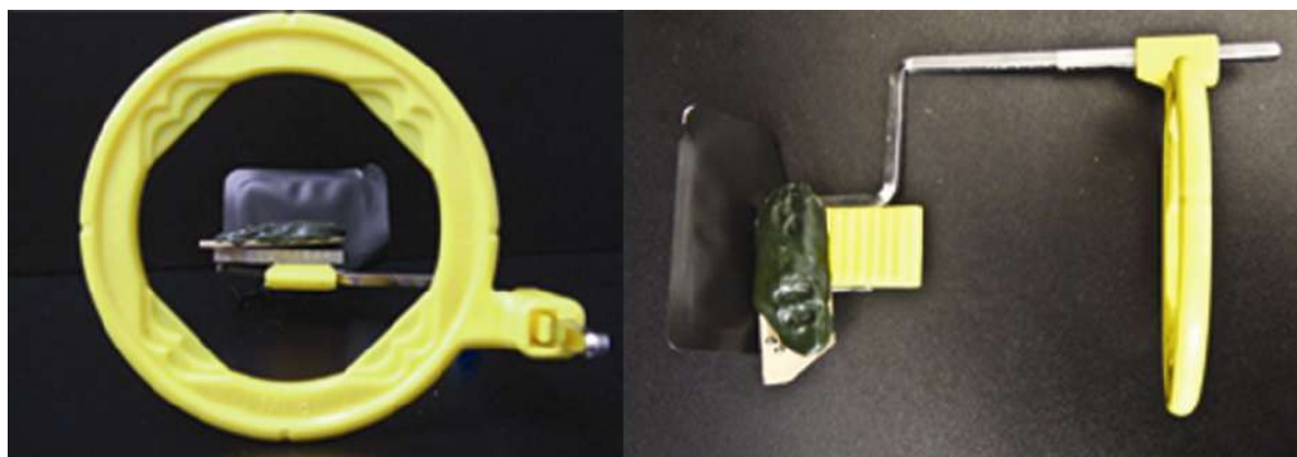
Figure 6.5: Individualized positioning device (adapted from the Rinn XCP position device, see Nackaerts et al 2006) for standardized follow-up radiography, using a film-holder with aluminum step wedge and occlusal key in green stent. Left image: Film-holder with occlusal green stent and phosphorplate positioned; Right image: Tube view of the device showing the occlusal stent, step wedge and phosphor plate.
