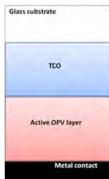
Figure 1.6: OPV architecture, where the TCO is deposited onto the glass support.
