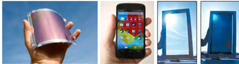
Figure 1.1: Solar panels, displays and electrochromic windows as applications for transparent conductive oxides.
