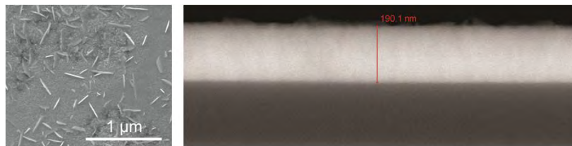
Figure 6.23: SEM and cross-sectional SEM image of 25 L of a 0.1 M Zn precursor deposited through spin coating (3000 rpm, 30 s and 1000 rpm/s). Each layer was treated on a hotplate at 200 °C in static air for 5 min.
