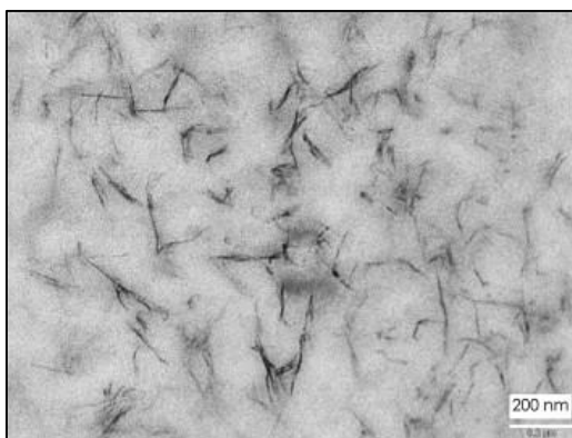
Figure 1-10: TEM image of a PHBV sample containing 5 wt% cellulose nanowhiskers [111]
