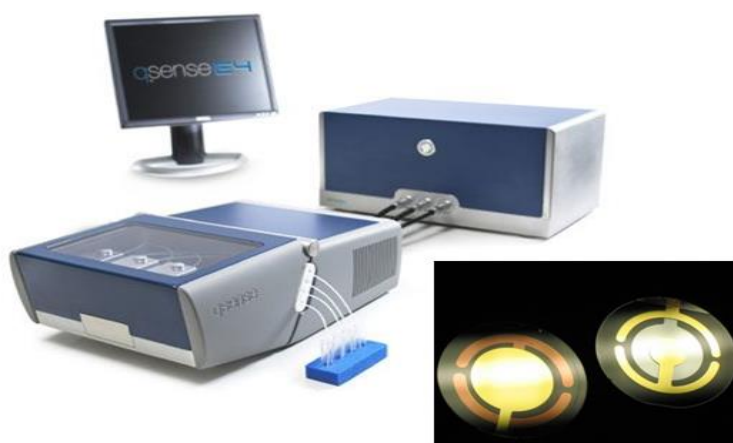
Figure 1.12 Quartz crystal microbalance with dissipation monitoring from Q-sense (Courtesy Q Sense, Biolin Scientific, Sweden)
