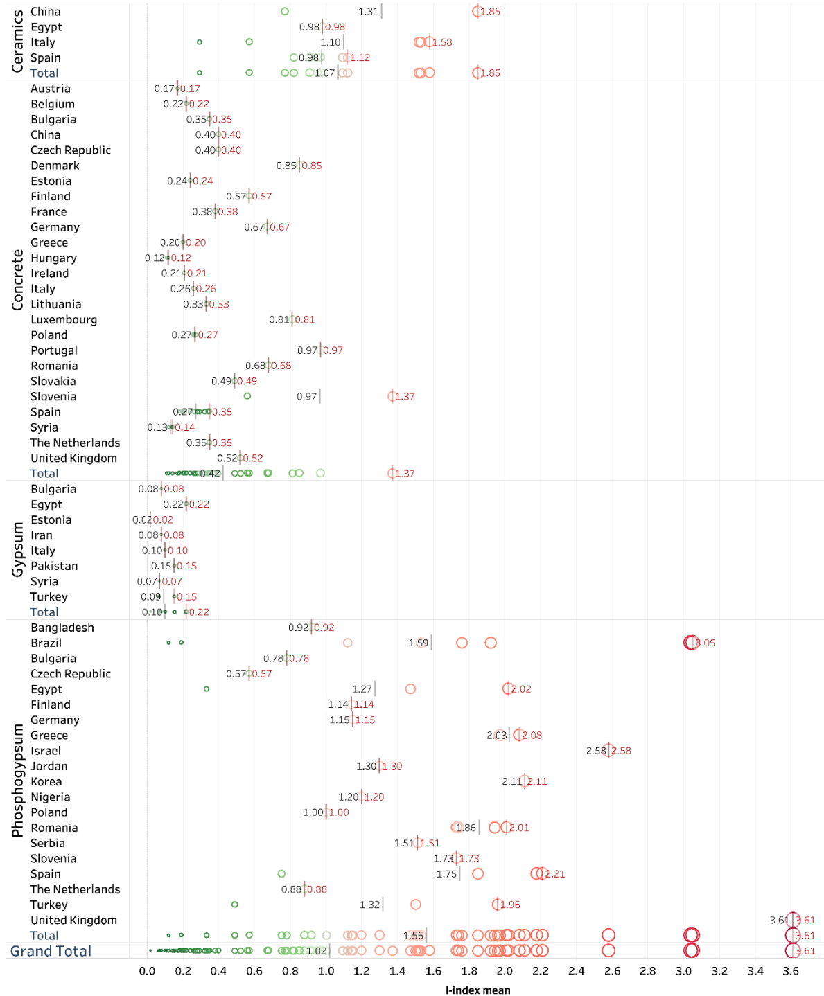
Figure 6 I-index (calculated from average reported activity concentrations) for building materials in different countries. Each circle is linked to a separate entry in the NORM4Building database. The average and maximal activity concentration for a given country are marked with respectively a black and red line (the numerical values are given).
