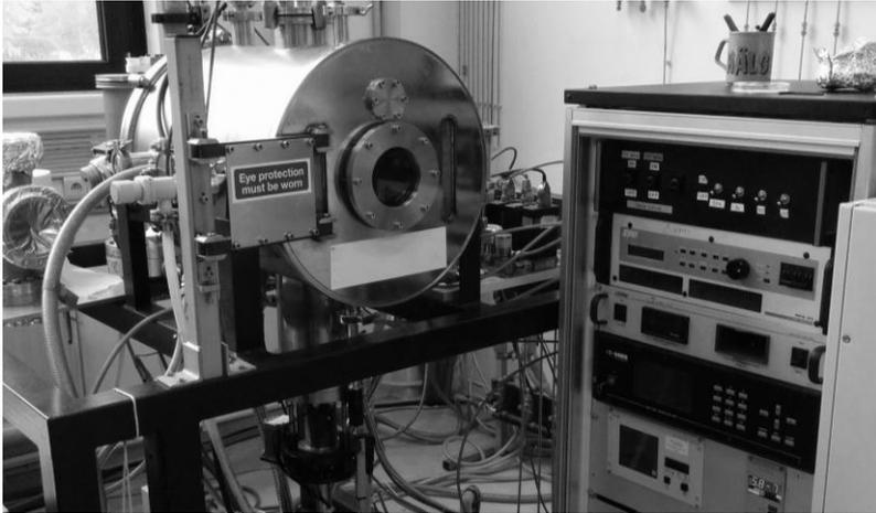
**Figure 3-3** – Image of home built system at IMO used for both sputtering and reactive-ion etching.
