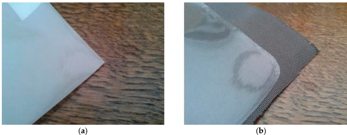
Figure 4. The textile substrate covered with PU (polyurethane) (a) or acrylate (b) to smoothen the textile roughness towards nm-range.
